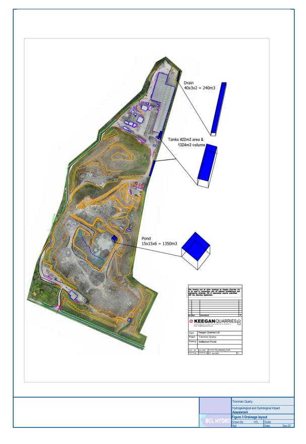
There is no natural baseflow in this drainage channel. It was excavated for the sole purpose of conveying water from the settlement tanks to the discharge point. The flow rate was and continues to be entirely dependent upon the discharge rate at the settlement tanks.
